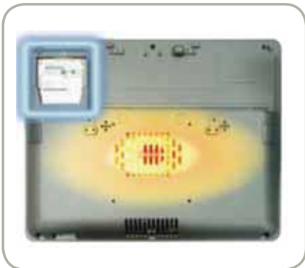
HDD isolated from main heat source on mother board
